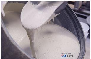
AALBORG EXCEL<sup>®</sup>, the 2nd UHPC premixed product, developed under the AALBORG INWHITE SOLUTION<sup>®</sup>, can satisfy manufacturers to seek the ultimate surface detailing and aesthetical expression, within aesthetic and architectural applications. The product is self-levelling and fast flowing, allowing combinations with pigments and fibers, achieving very smooth surface finishes, even with the most challenging shapes.
